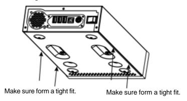
d) Replace the three screws which were removed in Step 1 from the back of the enclosure.
